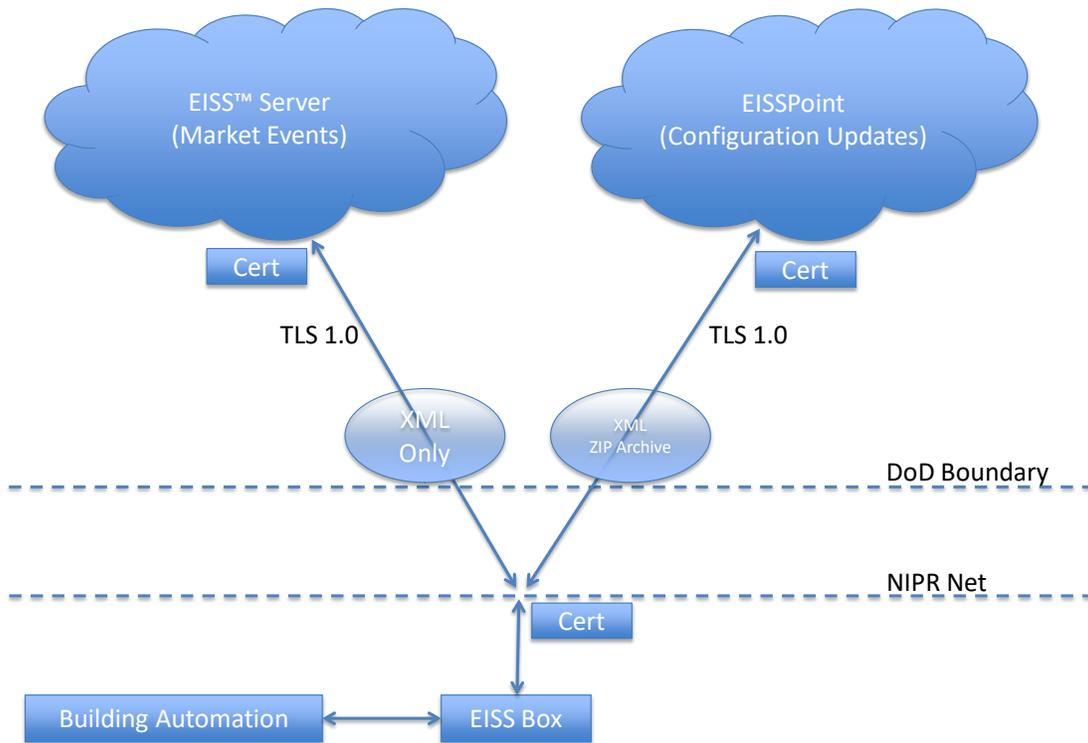
**Figure 2. EISS® Component Interaction Diagram**
