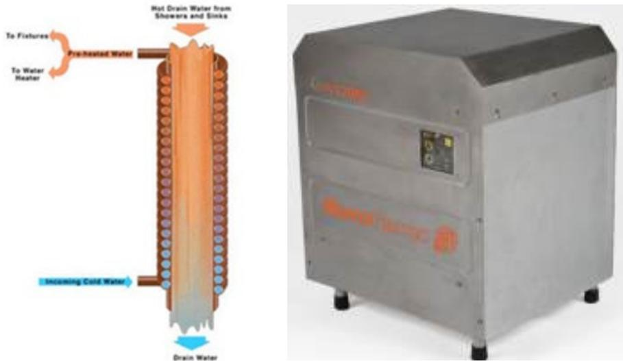
**Figure E1. GFX Schematic and Novothermic NVX2060 (L to R)**
