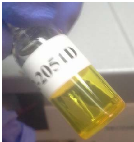
Figure 16. Solution obtained with 48% wt functionalized HTPB, 45% wt DOA and 7% wt isophorone cyclooctyne at ambient temperature
