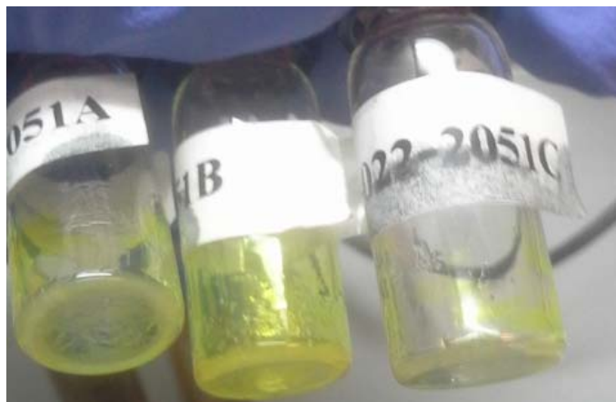
Figure 17. Picture of polymerization reactions of the different linked cyclooctynes with the functionalized HTPB after 16h at 50°C. Toluene diamine linker (left), hexamethylene diamine linker (middle) and isophorone diamine linker (right)
