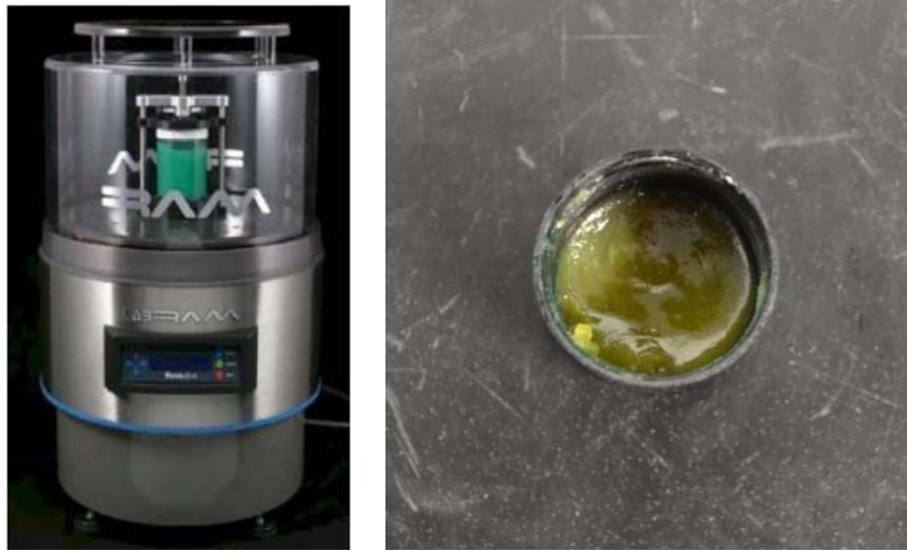
Figure 19. Picture of Resodyn LabRAM benchtop resonant mixer (left) and resulting propellant formulation with new binder system (right)
