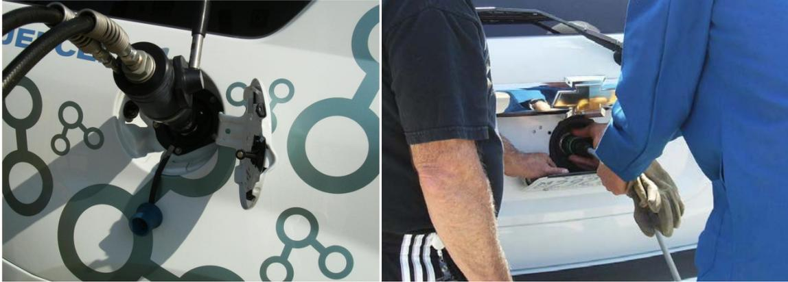
**Figure 5. Hydrogen fill and communication connections.** Shows the hydrogen fill connector (left) and the Type II communication connection (right).
