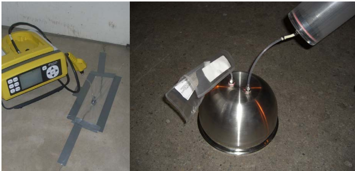
Figure 20: Examples of Vapor Entry Point Isolation and Testing
