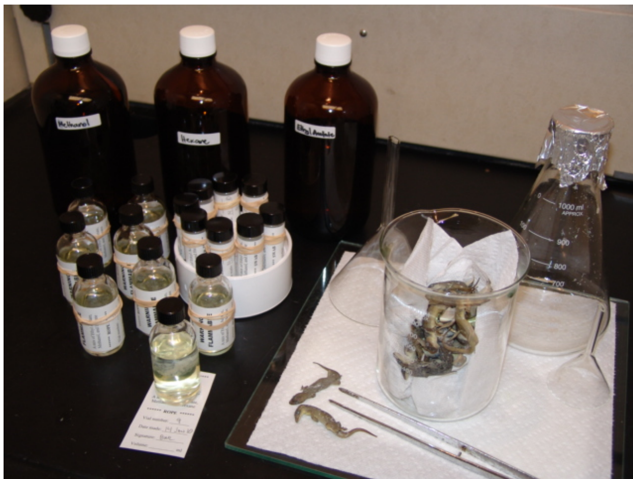
Figure 2. Chemical compounds present on the surface of dead geckos were extracted by immersing them in a mix of organic solvents.
