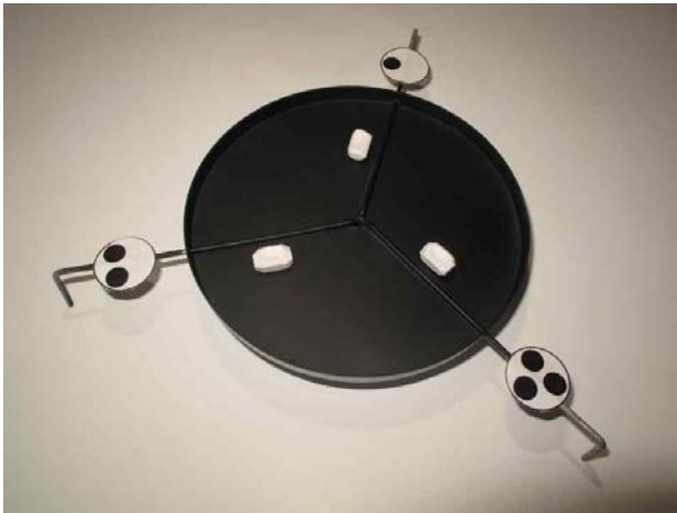
Figure 5. Differently scented bait matrices (or un-scented controls) were simultaneously offered to snakes on a Petri dish that was suspended in the snake's cage 5 cm below the glass lid covering the cage. Because the bait matrices looked identical, we aligned them with the treatment-associated markers seen attached to the legs. This allowed us to determine from surveillance video (in infrared light) which of the bait matrices a snake interacted with.
