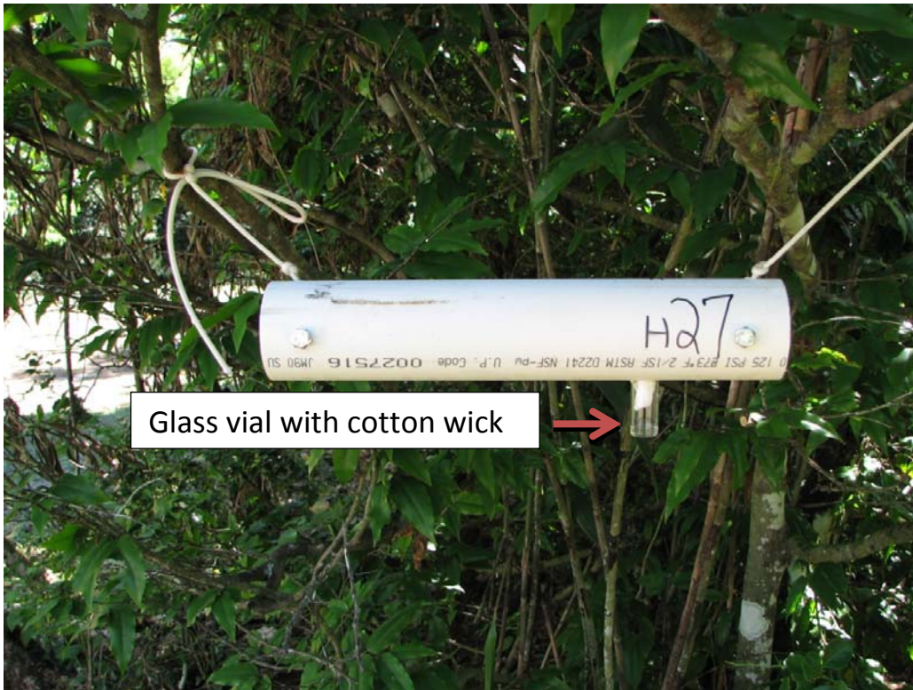
Figure 1. (Top) Standard bait station. (Bottom) Standard bait station modified with a glass vial and cotton wick for delivery of volatile chemicals inside the tube.
